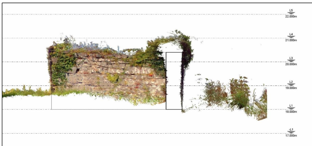
Sketch H: showing east elevation of South Transept. Vegetation treatment to be completed in Phase 1 and masonry works in Phase 2.
